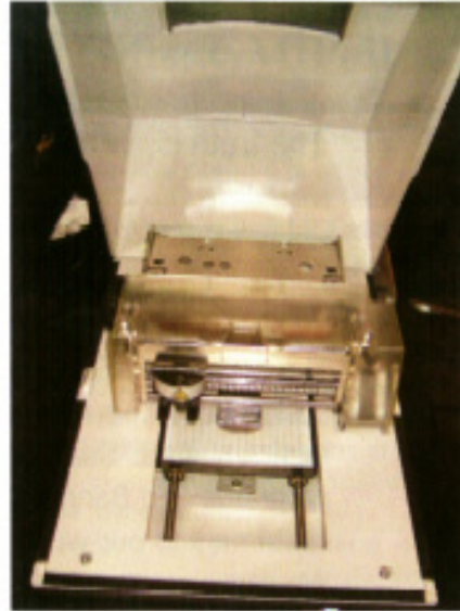
The Metaza printer takes a little over a square foot of counter space and has a drop down cover to reduce cutting noise
