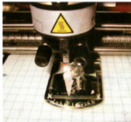
A self-adhering surface holds metal plates securely during the engraving process
